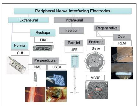
Figure 2. Classification of the different types of peripheral nerve interface electrodes. Extraneural electrodes are either normal (cuff)<sup>17-21</sup> or deform the nerve (FLAT),<sup>25</sup> while minimally invasive. Penetrating electrodes are inserted either perpendicular (USEA)41,42 or parallel (TIME)39 to the nerve axons. Those that require complete transection of the nerve have either enclosed electrodes (Sieve)<sup>43–46</sup> or open architecture (REMI).<sup>53</sup>
